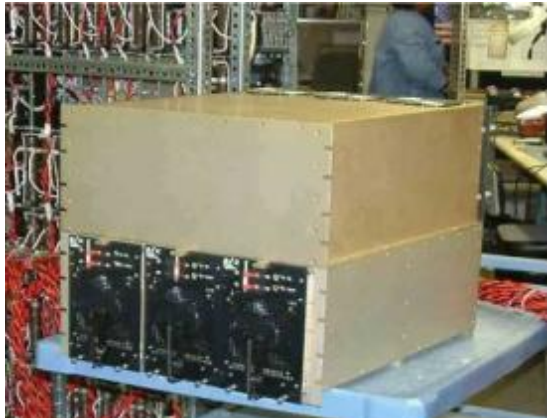
Power Supply for Solid State RF T/R Modules
